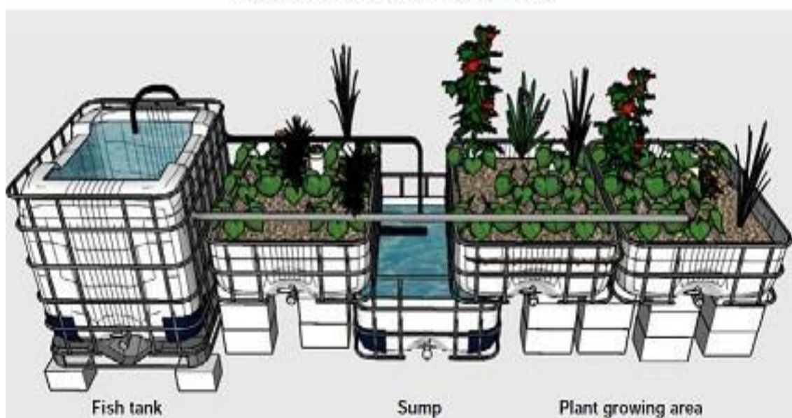
Illustration of a small media bed unit
